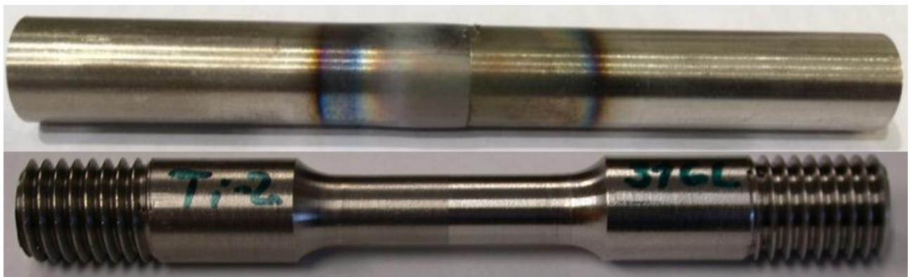
Fig. 6 Diffusion welded sample, T = 860^\circ\text{C} ; F = 0.5\text{kN} ; t = 40\text{min} performed in the argon shielding gas and testing sample machined from this workpiece
