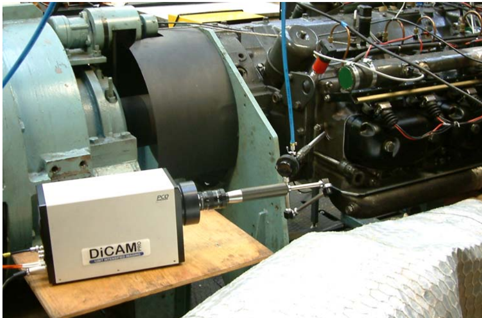
Fig.2: View of the cooled endoscope with camera connected by means of an optical link
