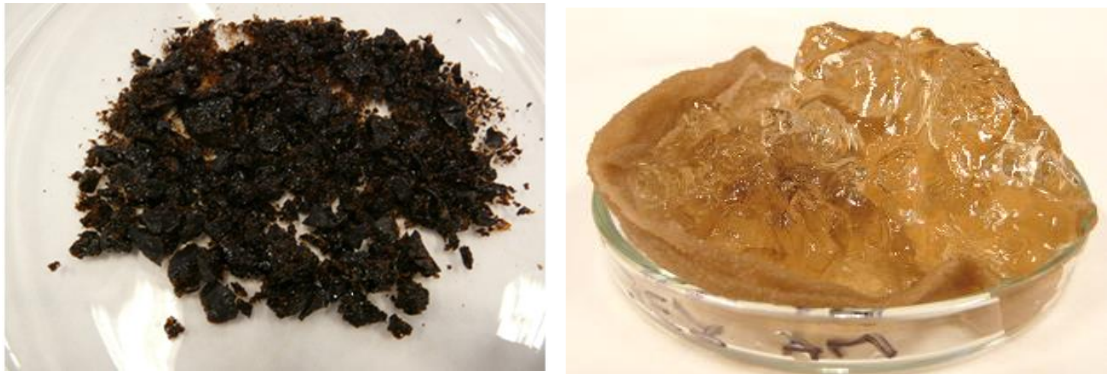
Figure 1 a) Xerogel of superabsorbent polymer. b) Swollen superabsorbent polymer.
