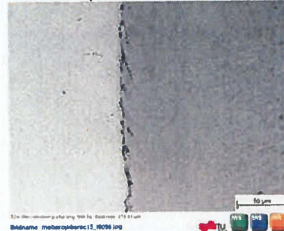
Figure 4. Microstructure of the sample performed at 950 °C, 40 minutes and - 0.5 kN.
