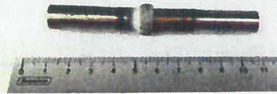
Figure 2. Macro image of the sample performed at 950 °C, 40 minutes and - 0.5 kN.
