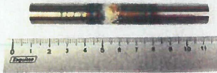
Figure 1. Macro image of the sample after the diffusion bonding; performed at 950 °C, 40 minutes and - 0.5 kN.
